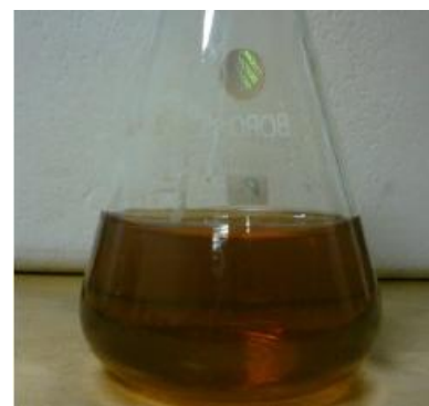
(C) Silver nitrate solution after adding 250µl of aloe vera extract and keeping at incubation in the dark for 24
